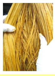
Existing module(SL), 28 m<sup>2</sup> (301 ft<sup>2</sup>) Packing density: 28.6% Without center distributor
